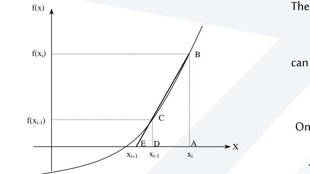
Figure 2 Geometrical representation of the Secant method.
